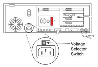
The Model 150 has an autoranging power supply, so you do not have to manually set the voltage switch.
