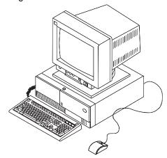
To power on the system, unlock the cover lock and slide the door to the left to access the white power switch.
