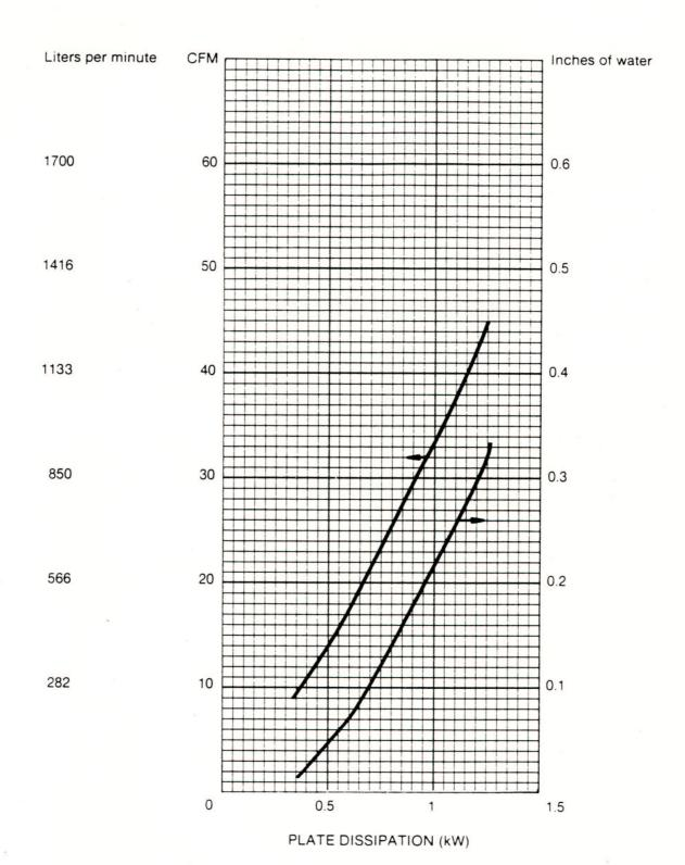
CFM and pressure required to keep anode temperature at 225°C.
